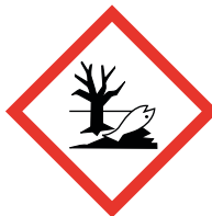
GHS 09 Hazardous to the environment
